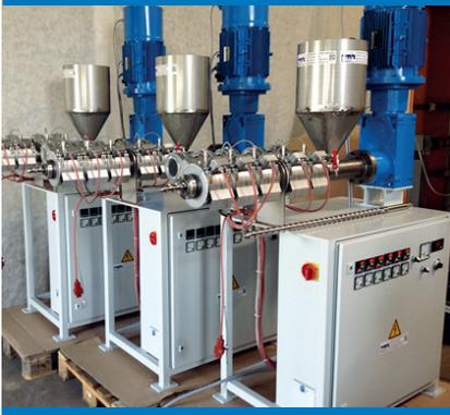
Extruder 30mm - 28d, AC-motor 7,5kW
