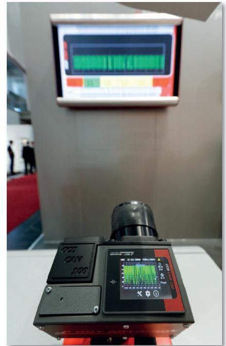
LAP GmbH Laser Applikationen, with which BST eltromat has worked in partnership for many years. The lasers from LAP are integrated in tire building machines, where projected laser lines are used to attain precise alignment of the individual rubber layers. At Tire Technology Expo 2019, BST eltromat will present the LASERmarker 1000, which, thanks to a fixed central laser, can make use of one or two moveable line lasers. This laser positioning system can be used just as flexibly.
