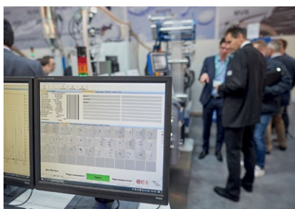
The OCS analysis software detects quality variations in real-time during the production process
