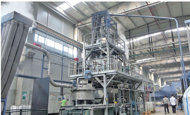
A centerpiece of the PET recycling plant is the hot washing step (All pictures: Futurapet/Herbold Meckesheim)
