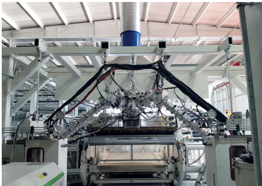
Co-extrusion set up of the board line at the entrance of the Multi-Touch roll stack
