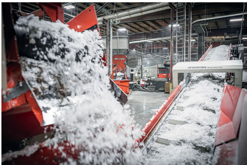
Five WEIMA single-shaft shredders shred plastic waste of all kinds
