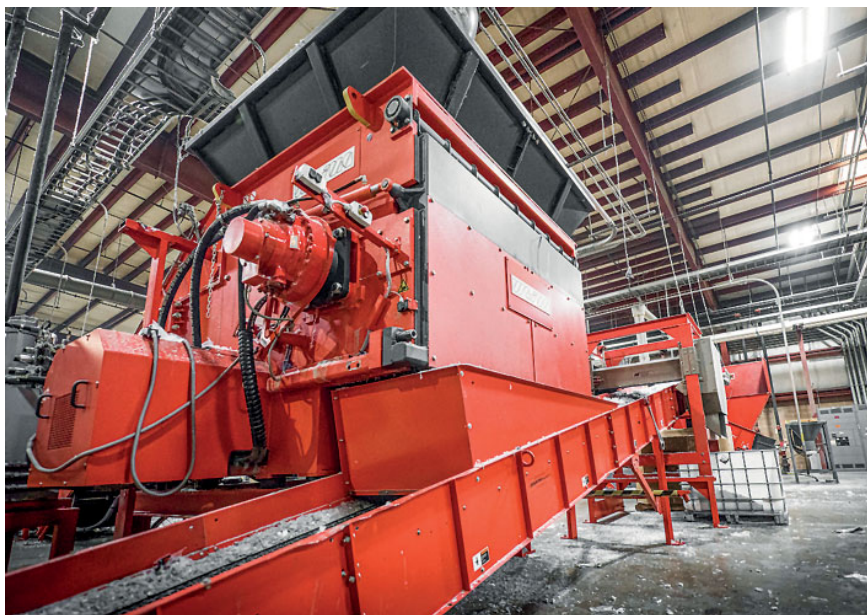
Five WEIMA single-shaft shredders shred plastic waste of all kinds
