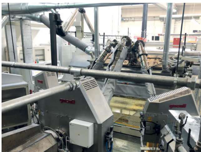
Sheet extrusion line at MP3 with three pressure- and process-constant Gneuss SFXmagnus melt filters
