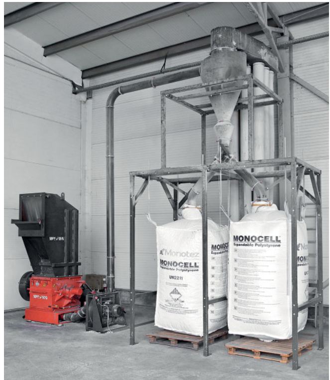
WEIMA WSM cutting mill with air extraction and big bags for regranulate collection
