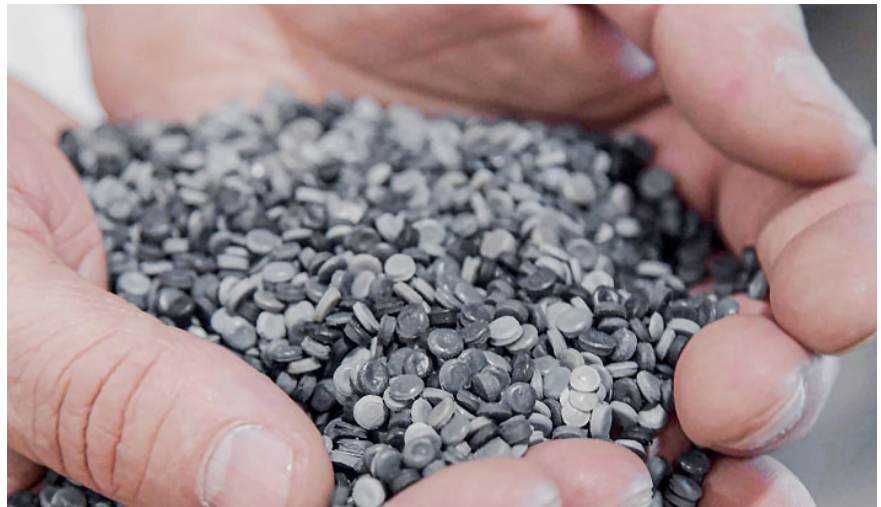
Fiberon regranulate from PE plastic waste
