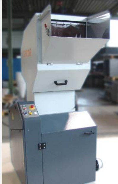
Photo 4: The RS 2404 B1 is designed for an hourly throughput of up to 160 kg and can be seen at the Fakuma stand of Getecha. This hopper granulator of the mid-market range is tailored to the use in blow-moulding plants
