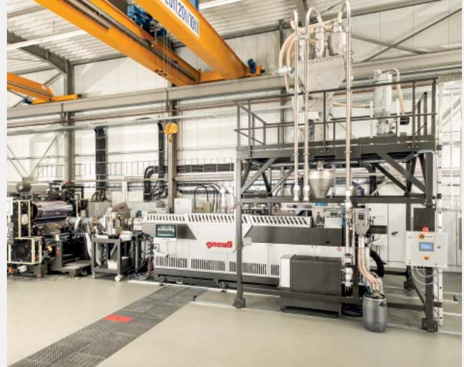
Sheet extrusion line with Multi Rotation Extruder MRS, Rotary Filtration System RSFgenius, and Online Viscometer VIS
