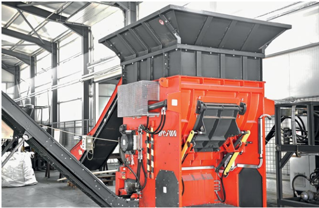
WEIMA W5.18 with wide inspection flap for the maintenance or removal of any impurities
