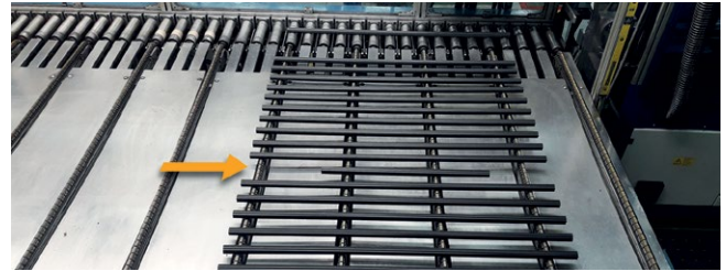
The new SawControl module, developed by PIXARGUS, makes profile cutting an integrated element of quality control. The software module performs two control functions for the cutting device: It sets the regular spacing for the continuous cutting process and cuts out defective profile portions at short lengths (Picture © COOPER Standard)
