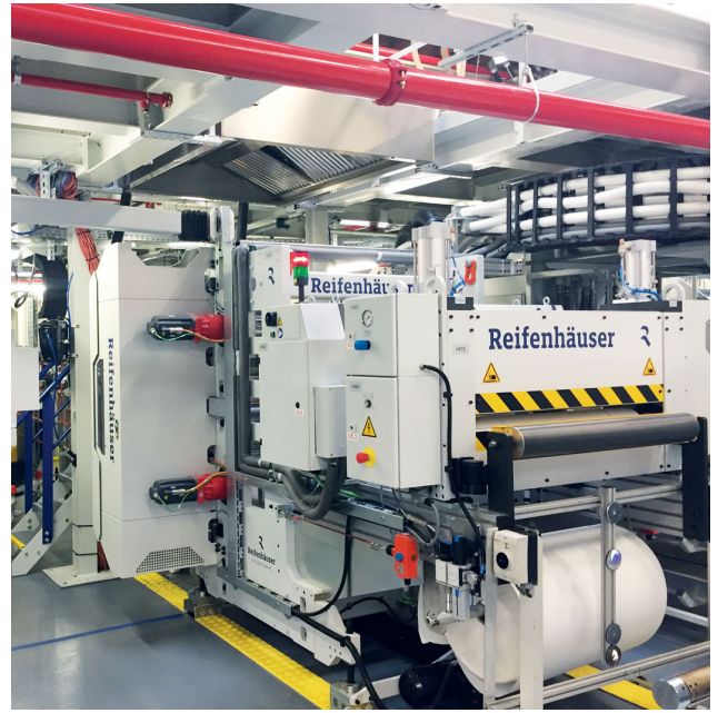
The mechatroni polishing stack MIREX MT from Reifenhäuser Cast Sheet Coating for barrier film applications (Photo: RPC Bebo Plastik)
