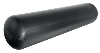
It is the inner skin of the tank. It absorbs the gas, surrounding the contents and sealing them off from the outside. The liner is subjected to high mechanical stresses and temperature ranges from -60 °C to +120 °C. Now, for the first time, the method developed by Kautex in cooperation with a plastics manufacturer enables hydrogen liners in sizes with industrial applications to be produced by blow molding.
