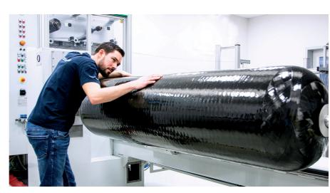
Prototype production in the Kautex Composite Center (All pictures © Kautex Maschinenbau GmbH)
