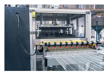
Virtually any common thermoplastic can be used to produce LFT pellets with reinforcement being provided as required by glass, steel, aramid or carbon fibers (photo: ProTec Polymer Processing)
