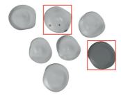
Contamination detected by optical camera
