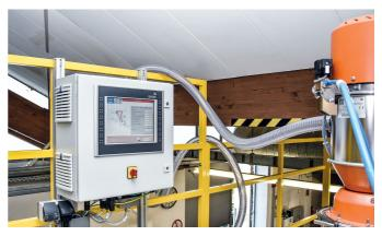
Pic. 1: Graviplus-series gravimetric synchronous dosing and blending station with four Labline dosing modules, one of which can be automatically supplied with material by a Metro conveying unit, while the other three have to be manually filled (all images: motan-colortronic)
