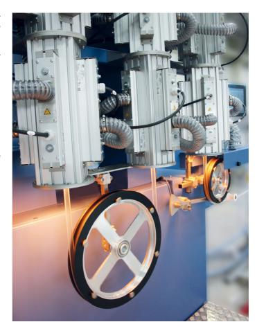
Picture 1: PEXLINK conveyor oven - 4-strand conveyor oven featuring a specifically designed guide and deflection system, a precondition for higher production speeds and higher outputs thanks to an extended residence time for each pipe dimension
