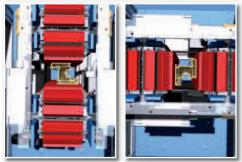
Haul off rotating 90° Slitting RB 2 with four sawing stations
