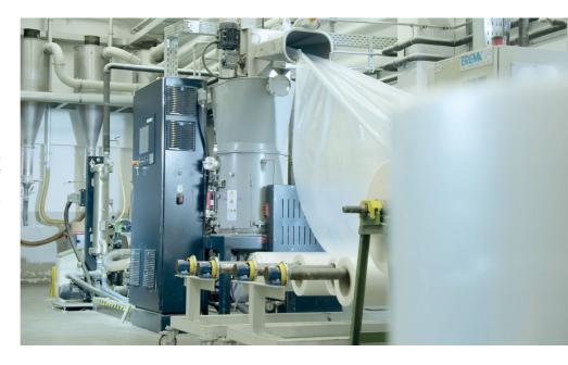
The INTAREMA® K at Coveris is in operation 24/7. 100 per cent of the recycled material is put back into the film production process.
