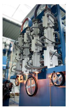
Picture 2: PEXLINK conveyor oven – Infrared units are the prerequisite for the optimum cross-linking of polyethylene. To protect the pipe from burining, a cooling system is part of the oven
