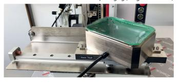
The 90° peel test on packaging is one of the most common tests in the field of food packaging. This type of test is used to determine adhesive/welding properties such as bond and tear strength. There are many peel and tear tests that use the same principle.
