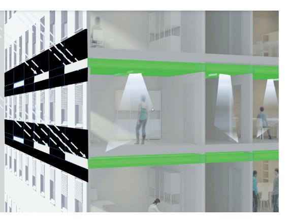
The daylight management system is based on the principle of light guidance and comprises three components: a film, a light shaft and light fixtures
