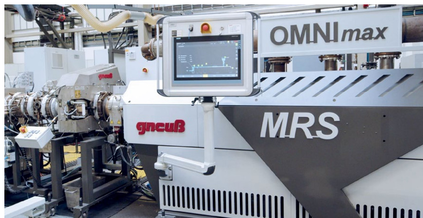
Gneuss OMNI max Recycling Machine with MRS extruder and RSFgenius filtration system
