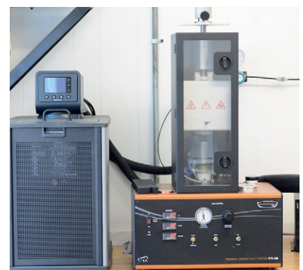
TA Instruments DTC-300 Thermal Conductivity Meter
