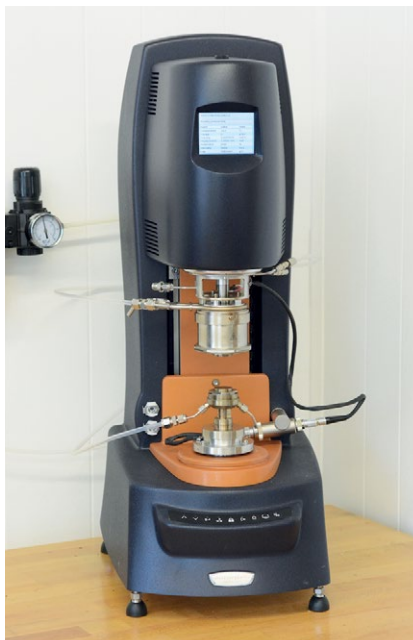
TA Instruments Discovery HR-2 Hybrid Rotational Rheometer
