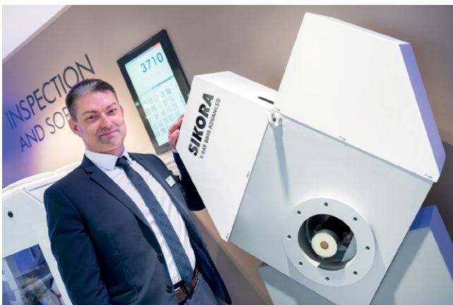
The X-RAY 8000 ADVANCED is used in CV lines for the quality control of cables
