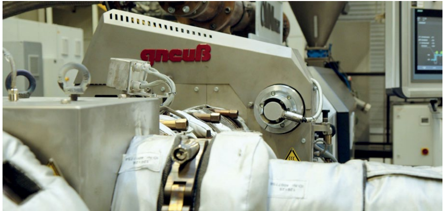
Patented Rotary Filtration System RSFgenius
